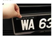
\*\* Please DO NOT place the sticker on chrome surface / metal surface / windscreen or near any metallic object. Metal will severely inhibit reading range.
