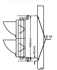
2) Fixed the traffic light to the pole with bolts and nuts.
